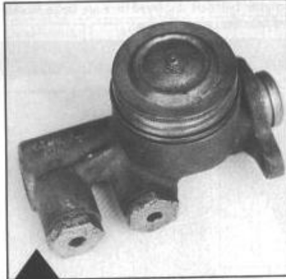
Casting No. E48327: The rarest in the set, the Z06 and J56 uses a special metallic brake and has a 1-inch bore with dual brake lines. The body is plated zinc dichromate, a yellow color, with a copper-plated cover. The inset photo notes the casting number E48327, which is located on the bottom with "Kelsey Hayes" prominently displayed.
