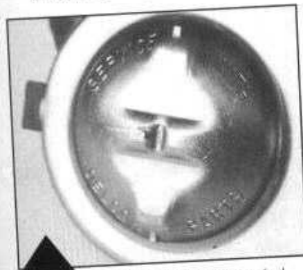
Casting No. 5480346: Like the '67 standard master cylinder, the cover is oval and plated zinc dichromate with an imprint saying "SERVICE WITH DELCO PARTS, USE DELCO SAE J1703 BRAKE FLUID." There is no tunnel between the two humps. The cover is held in place by two ball wires over each hump; the rear wire has a TG bail wire tag on it which is not shown here.
