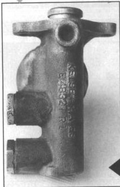
Casting No. E48327: The rarest in the set, the Z06 and J56 uses a special metallic brake and has a 1-inch bore with dual brake lines. The body is plated zinc dichromate, a yellow color, with a copper-plated cover. The inset photo notes the casting number E48327, which is located on the bottom with "Kelsey Hayes" prominently displayed.
