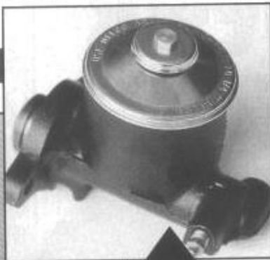
Casting No. 5462389—Power: Identical to the '63 without power, the distinguishing factor is the hex-head screw on the top to retain the cover as opposed to the thumbscrew. The photo (above right) notes the same casting number of 5462389.
