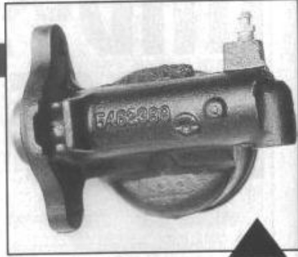
Casting No. 5462389—Power: Identical to the '63 without power, the distinguishing factor is the hex-head screw on the top to retain the cover as opposed to the thumbscrew. The photo (above right) notes the same casting number of 5462389.
