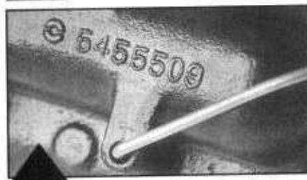
Casting No. 5455509: This master cylinder has a 1-inch bore and dual 1/4-inch brake lines that go to a steel block which serves as a low-fluid warning switch, not a proportioning valve. There are dual bleeder screws, one for each line. The body is painted semigloss black. The inset photo displays the casting number 5455509, which is located on the side of the master cylinder facing the engine.
