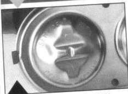
Casting No. 5455509: The cover is oval and plated zinc dichromate with an imprint saying "SERVICE WITH DELCO PARTS, USE DELCO SAE J1703 BRAKE FLUID." There is no tunnel between the two humps. The cover is held in place by two ball wires over each hump; the rear wire has a YA bail wire tag on it which is not shown here.
